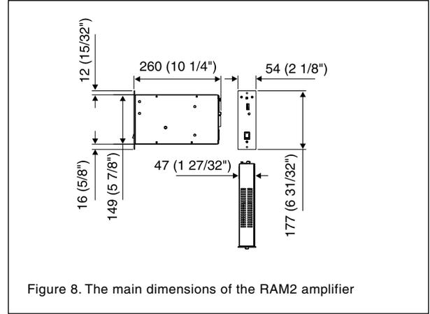
Figure 8. The main dimensions of the RAM2 amplifier
