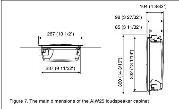
Figure 7. The main dimensions of the AIW25 loudspeaker cabinet
